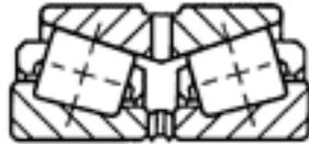
**Radial Tapered Cylindrical Bearing
